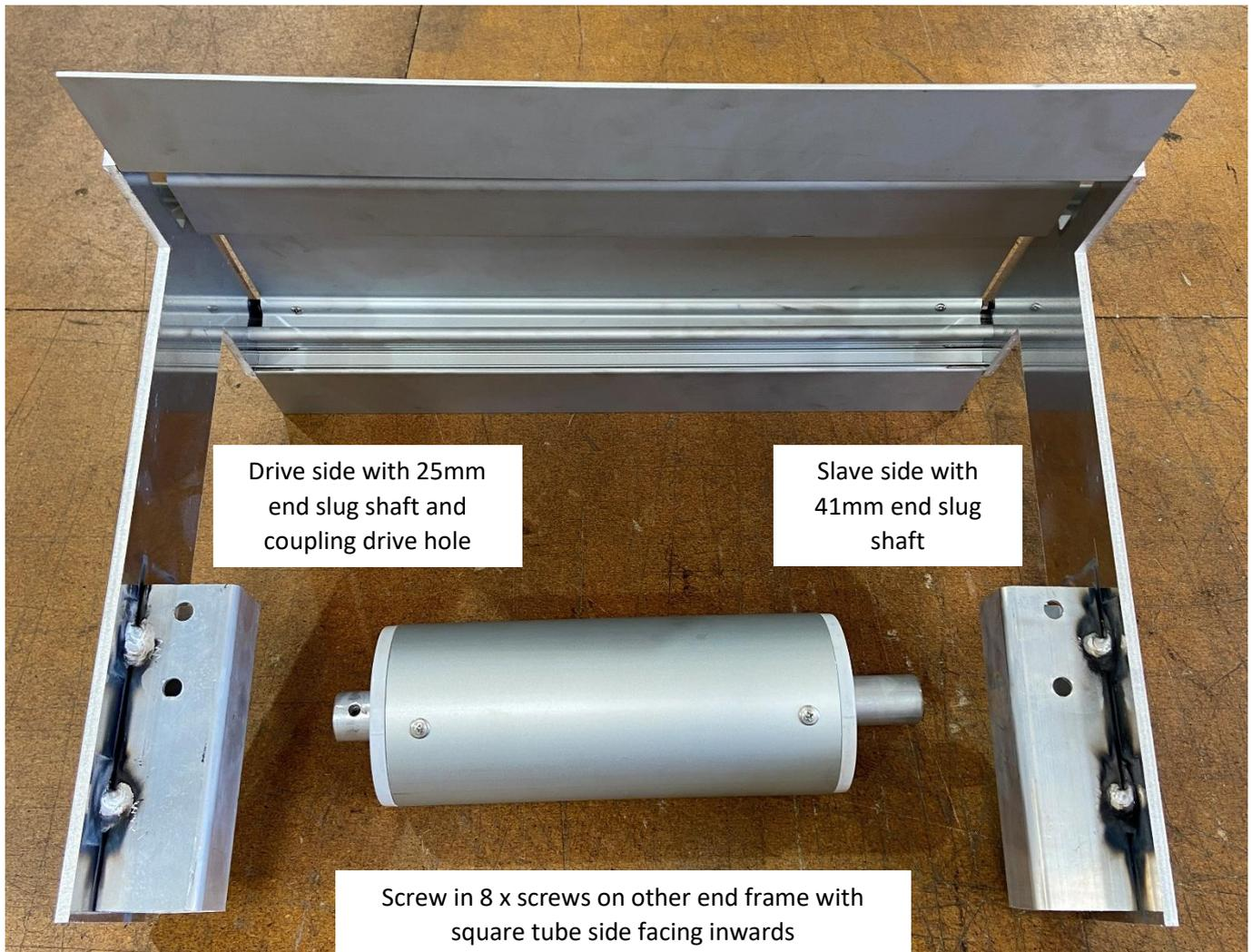
Connect gearbox drive coupling to 25mm end slug with hole through using 6mm bolt and nyloc nut
