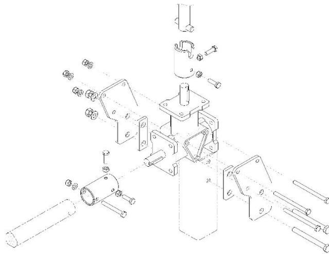
The roller Bevel Gearbox drive mechanism can be installed either side of unit. To change ends simply unbolt the 8mm mounting bolts (through square tube) to remove and turn the roller around
