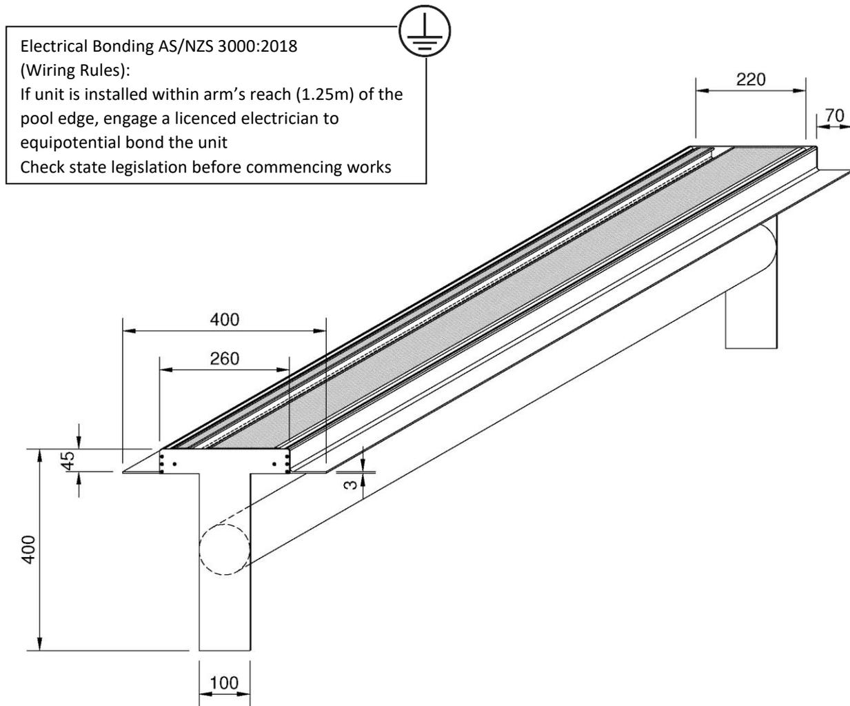
Length of DMR is to the outside of the unit. Prepare mounting for DMR to either sit on or be suspended under noting finished height of the unit should be finished paving/deck level
